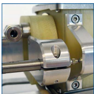
Unit for compression measurement (CMD) for fully automated compression measurement analysis
